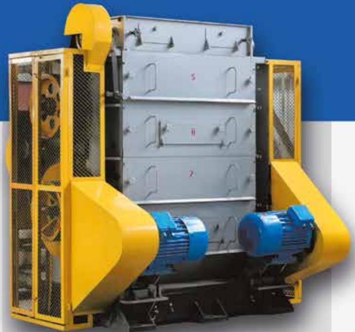
Roller mills are used for continuous mechanic crushing and flaking of seeds kernels of various oil plants.
